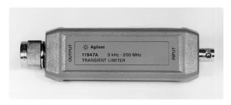
Frequency range Insertion loss Maximum input level 9 kHz to 200 MHz 10 dB Continuous: 2.5 W (+34 dBm) Pulse: 10 kW for 10 µsec DC: ±12 V
